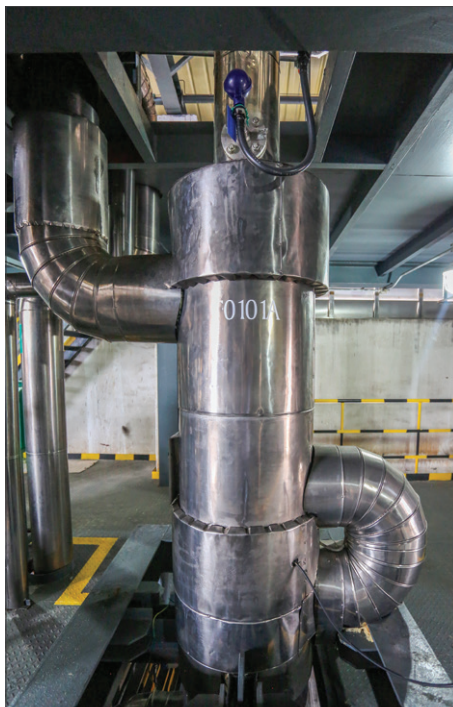
Fig. 7 - Top end of the 7.50 m long Miprowa ® Reactor installed at Shaoxing Eastlake High-Tech in China with connectors for heat transfer medium
