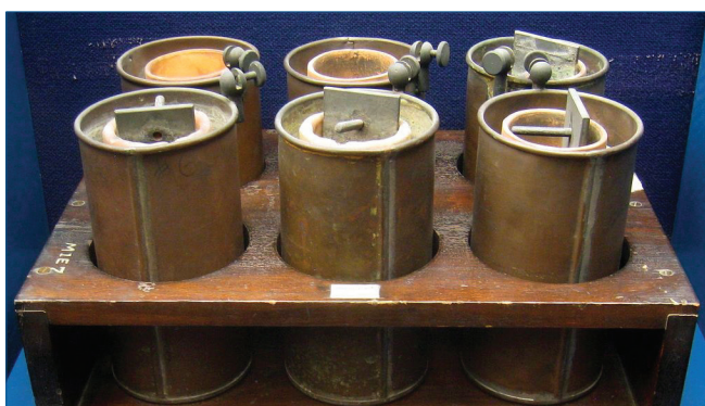
Pile di Daniell in batteria, 1836 (National Museum of American History, Washington, DC, USA)
